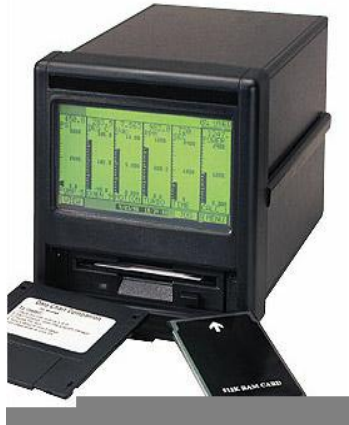
Figure 7.7. Videographic recorder with magnetic storage media (PCMCIA card or floppy disk)
